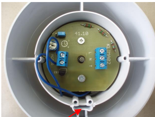
Place for service cable
