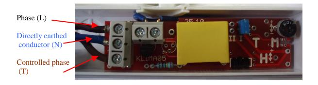
3. Fan's electronic allows speed control and airflow control, what's more save energy. Carefully turn potentiometer M with small screwdriver directions +-. Regulation is possible only if there is power supply on terminal T (switch ON on-off switch), otherwise device runs maximum speed. You can controll fan's speed in steps - 50%, 70%, 85% and 100%.
