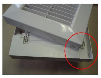
Turn ON on-off switch to bring power supply 230V/50Hz into device – <u>Warning!</u> device start to work (according to set parameter M) only if thermoactuator gets warm and opens the shutter – after cca 40 seconds. Turn OFF on-off switch to disconnect power supply – fan stop works.
