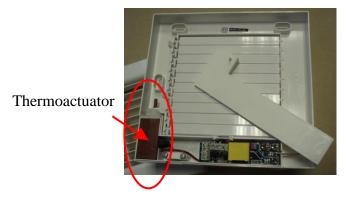
Turn OFF on-off switch to disconnect power supply – fan stop works according to set parameters, thermoactuator gets colder and closes the shutter (cca 1,5 minutes until shutter is fully closed).
