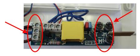
If *shutter* does not work properly, <u>disconnect power supply</u> and controll connection of thermoactuator and motor cable into terminal strip – they are connected together.
