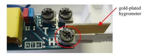
5. Fan's electronic allows speed control and airflow control, what's more save energy. Carefully turn potentiometer (**M**) with small screwdriver directions +-. Regulation is possible only if there is power supply on terminal T (switch ON on-off switch), otherwise device runs maximum speed. You can controll fan's speed in steps - 50%, 70%, 85% and 100%.
