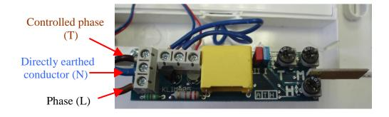
3. Carefully turn potentiometer (**T**) in clockwise direction with small screwdriver from 30 seconds to 30 minutes (directions +-). For exact time experimentally turn and try.
