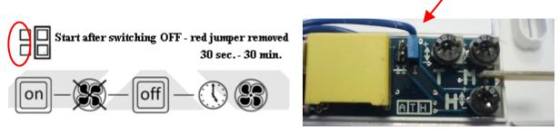
4. Device has got a hygrometer on electronics, which allows setting of humidity level. Carefully turn potentiometer (**H**) to set level of relative humidity, from which will device start to work (from 50% to 90% - relative humidity means where the fan is mounted).
