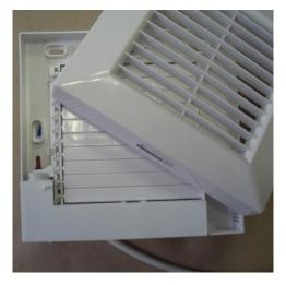
4. Turn on on-off switch to bring power supply 230V/50Hz into device – fan starts to work. At the same time termoactuator gets warmer and during cca 50 seconds is the shutter open. After switch off device stops. Thermoactuator get colder and closes the shutter (watt cca 2,5 minutes until complete closure).
