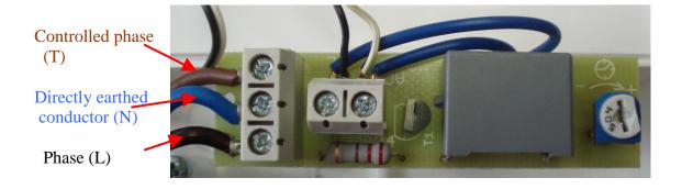
3. Carefully turn potentiometer in clockwise direction with small screwdriver from 30 seconds to 25 minutes (directions +-). For exact time experimentally turn and try. Only after switching OFF on-off switch (no power supply on T) overrun starts. After set time the device stops.
