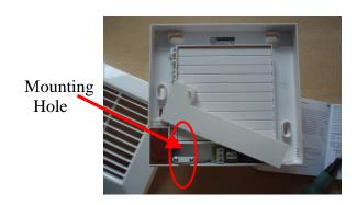
2. Connect the fan with power supply using the terminal strip. Usually goes from wall electric cable with 3 wires, so the blue is directly earthed conductor (N), brown / black is the phase conductor (L – under constant voltage) and third yellow-green is the circuit protective conductor (no need to connect when mounting plastic fan, can be blinded). Install the fan so the service cables will be in lower part of the fan.
