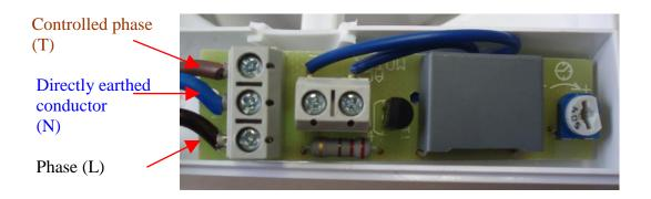
3. Carefully turn potentiometer in clockwise direction with small screwdriver from 30 seconds to 25 minutes (directions +-). For exact time experimentally turn and try. Only after switching OFF on-off switch (no power supply on T) overrun starts. After set time the device stops.
