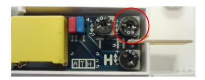
5. Device has got a hygrometer on electronics, which allows setting of humidity level. Carefully turn potentiometer (**H**) to set level of relative humidity, from which will device start to work (from 50% to 90% - relative humidity means where the fan is mounted).
