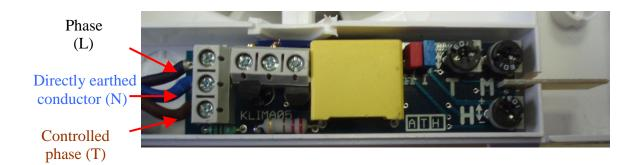
3. Carefully turn potentiometer (**T**) in clockwise direction with small screwdriver from 30 seconds to 30 minutes (directions +-). For exact time experimentally turn and try.
