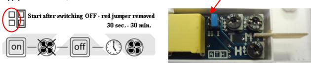
4. Fan's electronic allows speed control and airflow control, what's more save energy. Carefully turn potentiometer (**M**) with small screwdriver directions +-. Regulation is possible only if there is power supply on terminal T (switch ON on-off switch), otherwise device runs maximum speed. You can controll fan's speed in steps - 50%, 70%, 85% and 100%.
