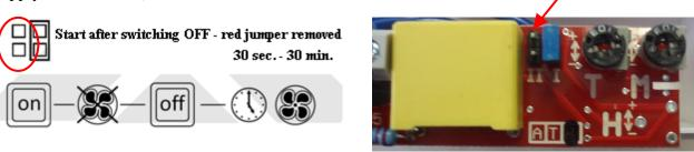
4. Fan's electronic allows speed control and airflow control, what's more save energy. Carefully turn potentiometer **M** with small screwdriver directions +-. Regulation is possible only if there is power supply on terminal T (switch ON on-off switch), otherwise device runs maximum speed. You can controll fan's speed in steps - 50%, 70%, 85% and 100%.
