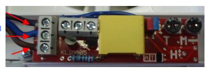
3. Carefully turn potentiometer (**T**) in clockwise direction with small screwdriver from 30 seconds to 30 minutes (directions +-). For exact time experimentally turn and try.
